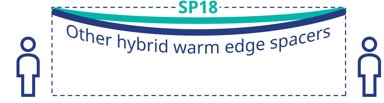
Enhanced profile stability due to increased steel wire diameter during the entire production process
