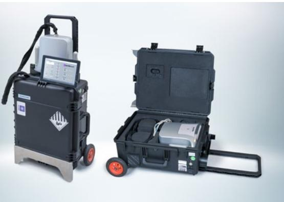
The Sparklike Laser Portable™ is impressively compact and easy to handle. It can be easily used to measure noble gas content virtually anywhere.
